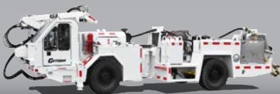
SHOTCRETE SPRAYING & TRANSPORT
